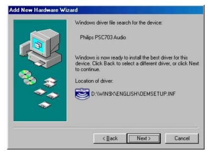
5. Windows<sup>®</sup> then copies the files. You may be prompted to insert your Windows<sup>®</sup> CD or floppy, as the core sound components of the operating system may need to be copied as well. These include audio Codecs, the Mixer and the Sound Recorder program.
